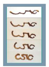
New smart elastomeric materials with thermal stimuli response An elastomeric material formed by interpenetrated ionic and covalent networks with shape memory effect which allows to respond to thermal stimuli.
